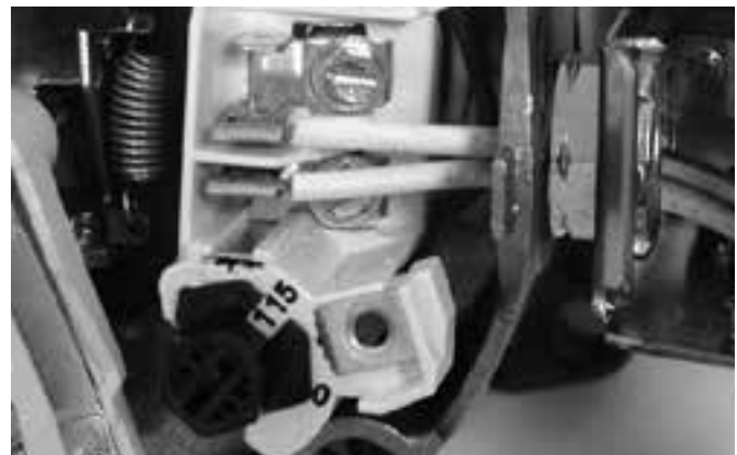
Figure 11: Voltage set to 115 V, Dial Type
